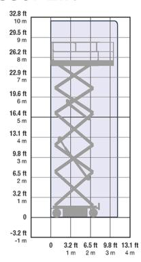
Working Height 9.92m Max Platform Height 7.92m Safe Working Load 227kg 2.15m Height Height - Guardrails Lowered 1.91m Length x Width 2.32m x 0.81m Deck Size 2.13m x 0.71m Deck Size Extended 3.04m x 0.71m Weight 1890kg Tyres Non-marking
